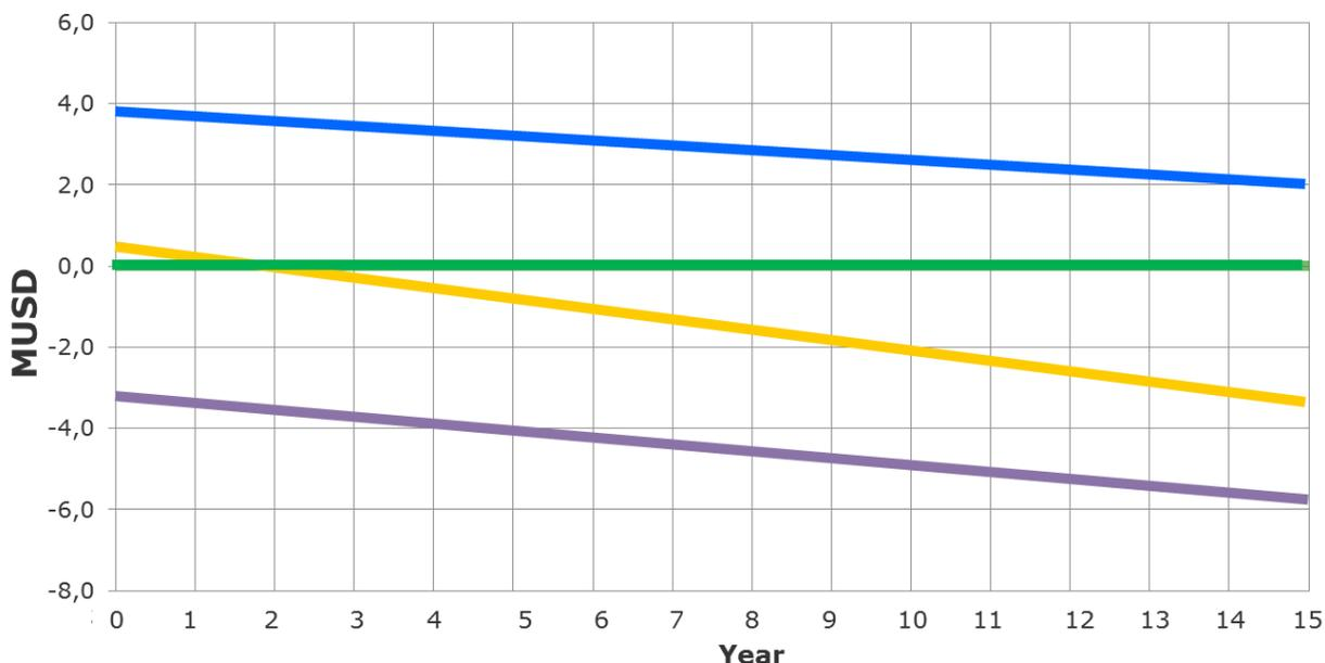
**Figure 1 - Combined cumulative discounted costs (capex and opex) in MUSD, comparing different arrangement designs and emission compliant technologies. All economic figures are relative to the green line which is the base case. The results are project specific subject to the operating profile of the vessel, not valid for general statements.**
