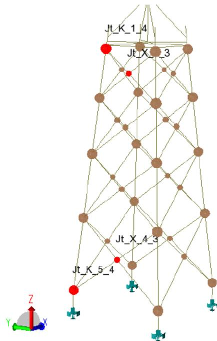
Figure 3: Selected result locations Jt\_K\_5\_4 and Jt\_X\_1\_3 within the jacket.
