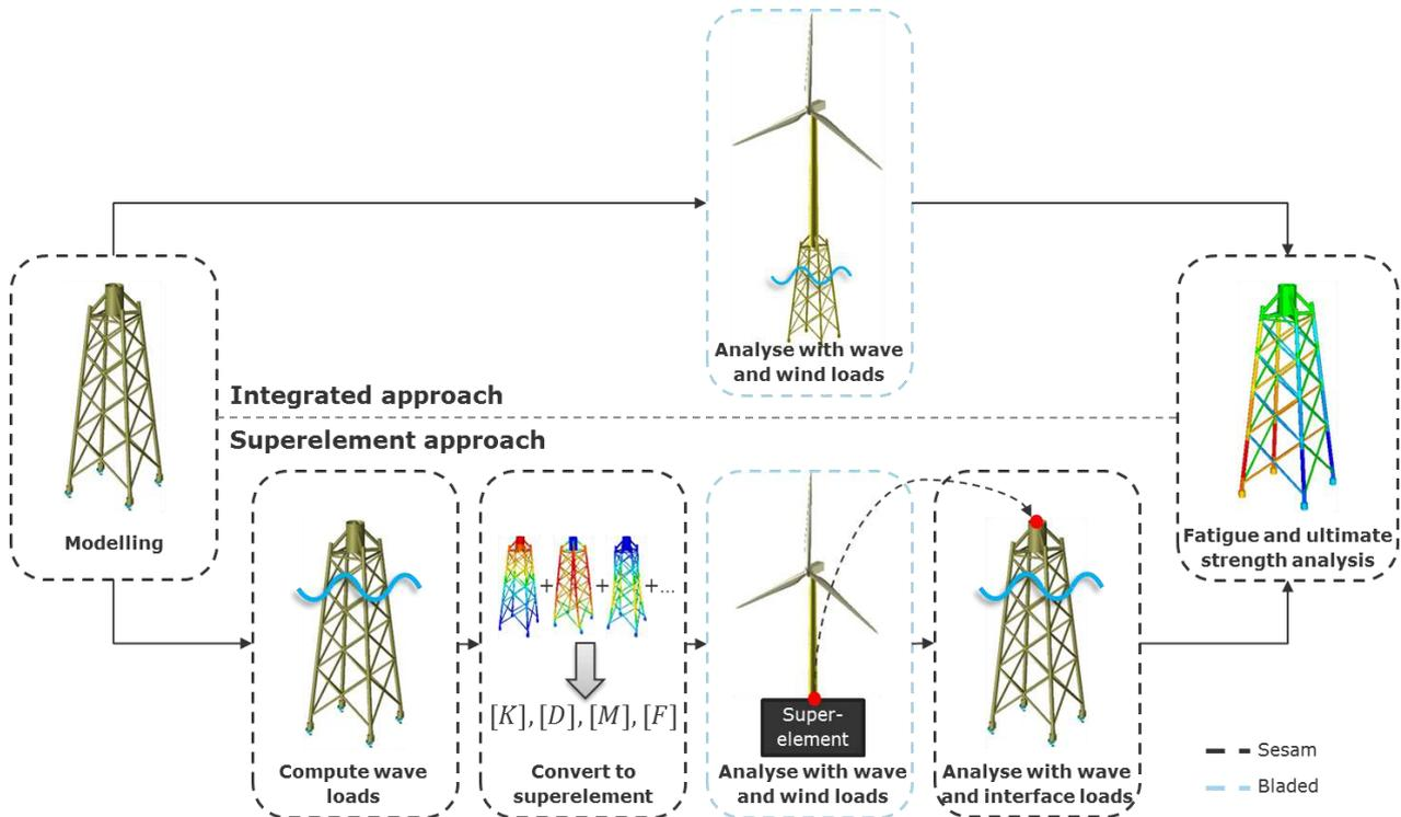
Figure 1: Visualization of the integrated and superelement workflows.
