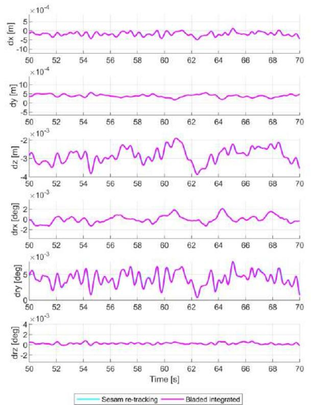
Figure A.6: Displacements and rotations at joint Jt\_K\_5\_4.
