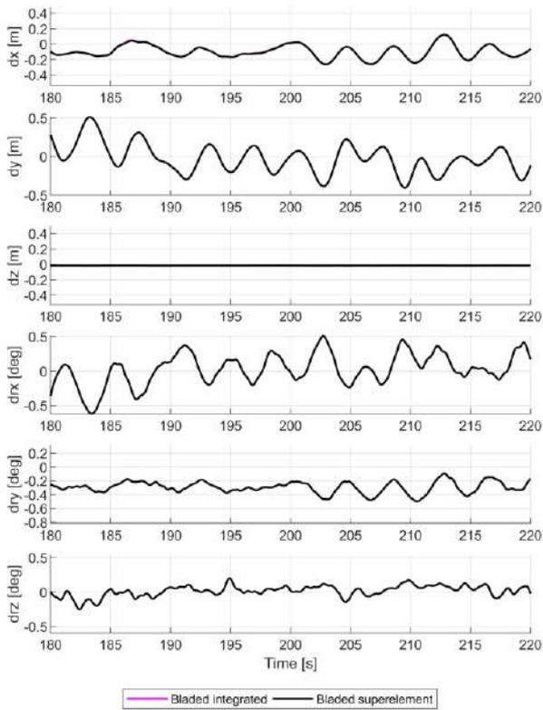
Figure A.12: Displacements and rotations at the tower top.
