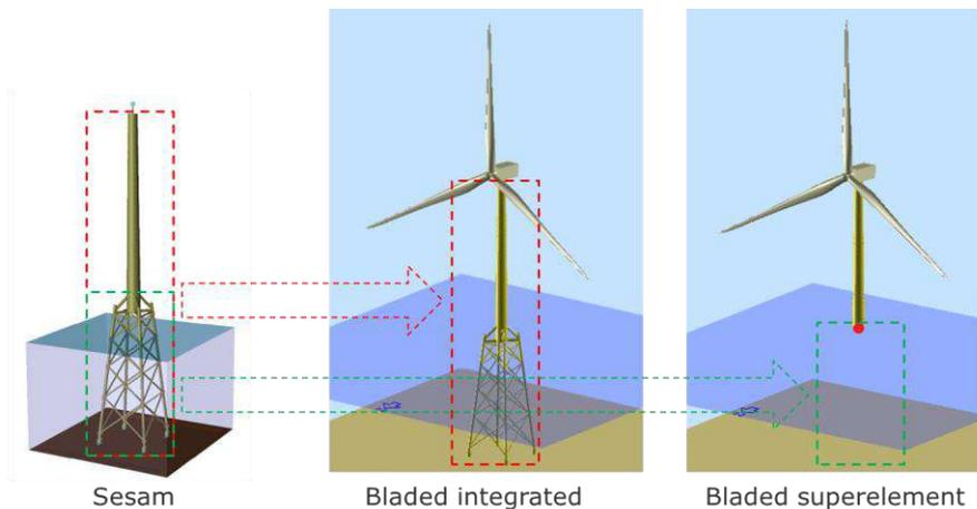
Figure 2: Left: complete structure including jacket and tower and point mass RNA in Sesam. Middle: jacket and tower from Sesam combined with wind turbine in Bladed. Right: superelement from Sesam combined with wind turbine in Bladed.
