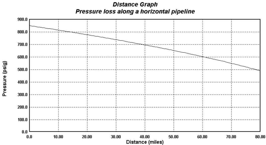
**Figure 1** - Steady-state pressure profile -- P1 = 850 psig
