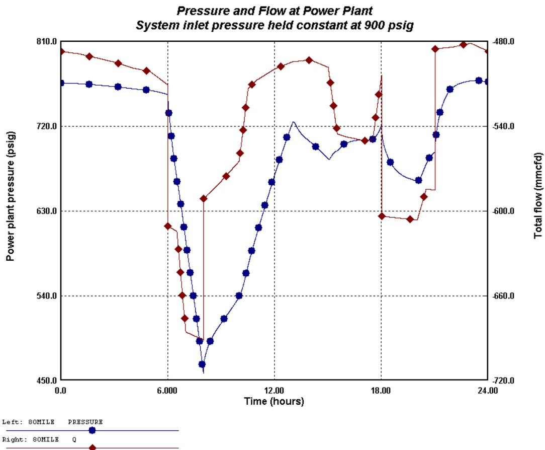
**Figure 9** - Pressures and flow changes due to increases source pressure
