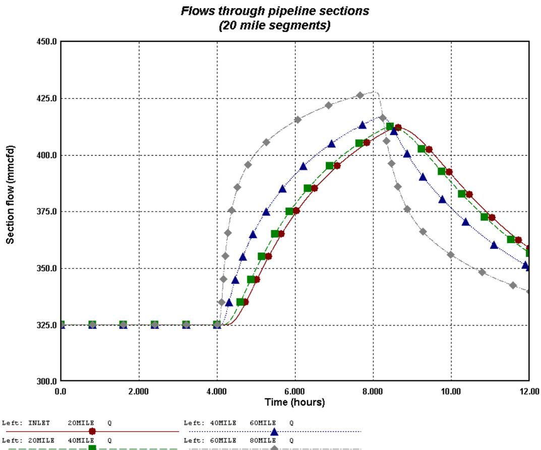
**Figure 6 - Flows along the pipeline, shown in 20-mile segments**
