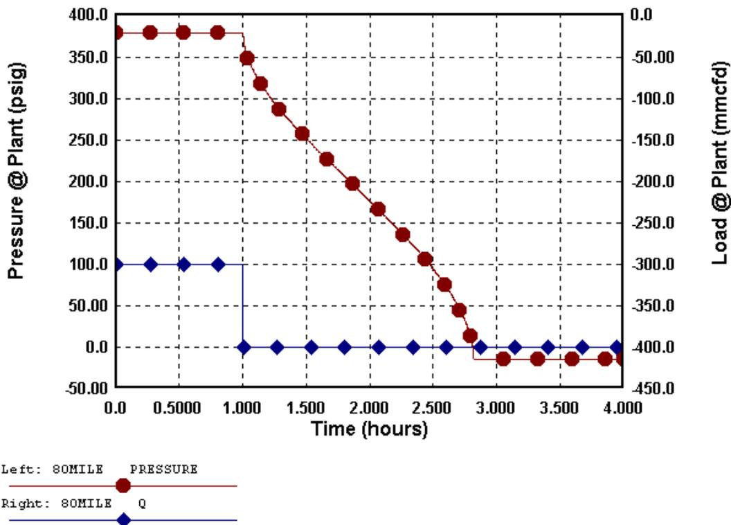
**Figure 10 - Gas Controller Problem -- Transient Analysis of Full Turbine Load with 750 psig Inlet**
