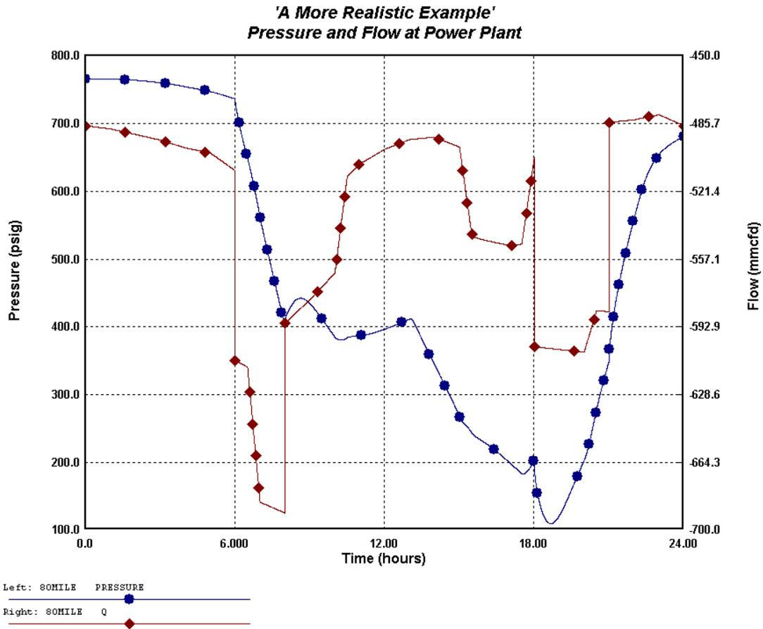
**Figure 8** - Complex load interaction and resultant pressures at power plant
