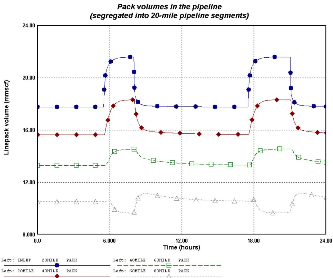
**Figure 6 - System pack volume response along the pipeline**
