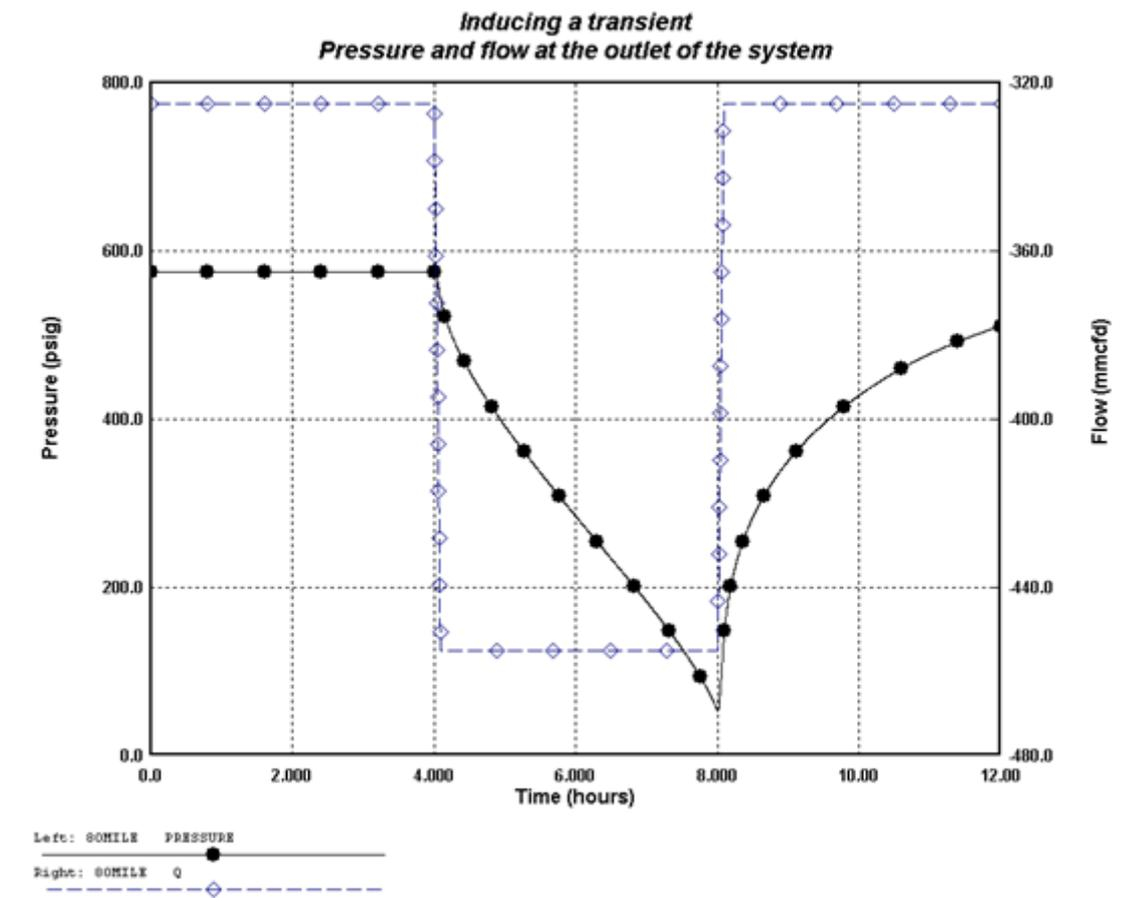
**Figure 4** - Pressure (left axis) and Flow (right axis) at the end of the pipeline
