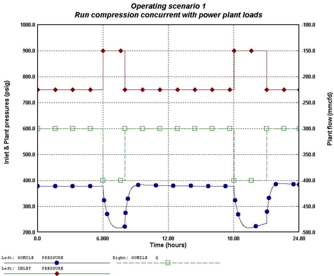
**Figure 4 - Gas Controller Problem -- Operating Compressors with Power Plant Flows**
