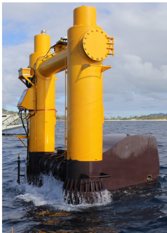
Figure 15. Energy Department-supported 'Azura' wave energy converter is installed at a U.S. Navy test site in Hawaii. Photo courtesy of Northwest Energy Innovations. Source: https://www.energy.gov/articles/capturing-motion-ocean-wave-energy-explained
