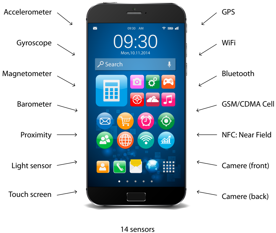
Figure 2. A “Smart Phone” integrated with fourteen types of sensors. [Image Credit 1]
