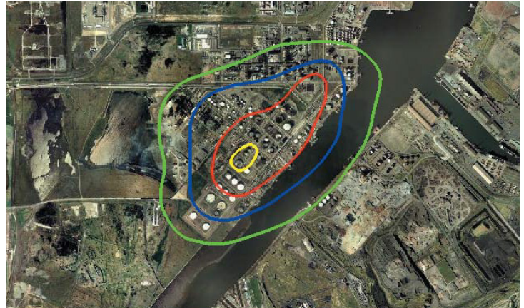
Aerial photograph of a chemical plant including individual risk shown as iso-contours
