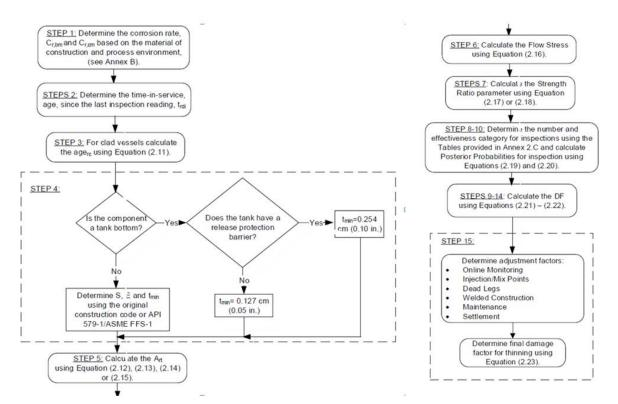
Figure 3: Thinning damage factor calculation procedure in API RP 581 3rd edition
